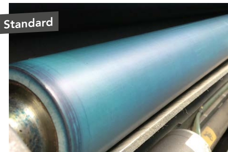
Soiling degree of a standard metering roller in comparison to the PERLADAMP after a complete daily production.
