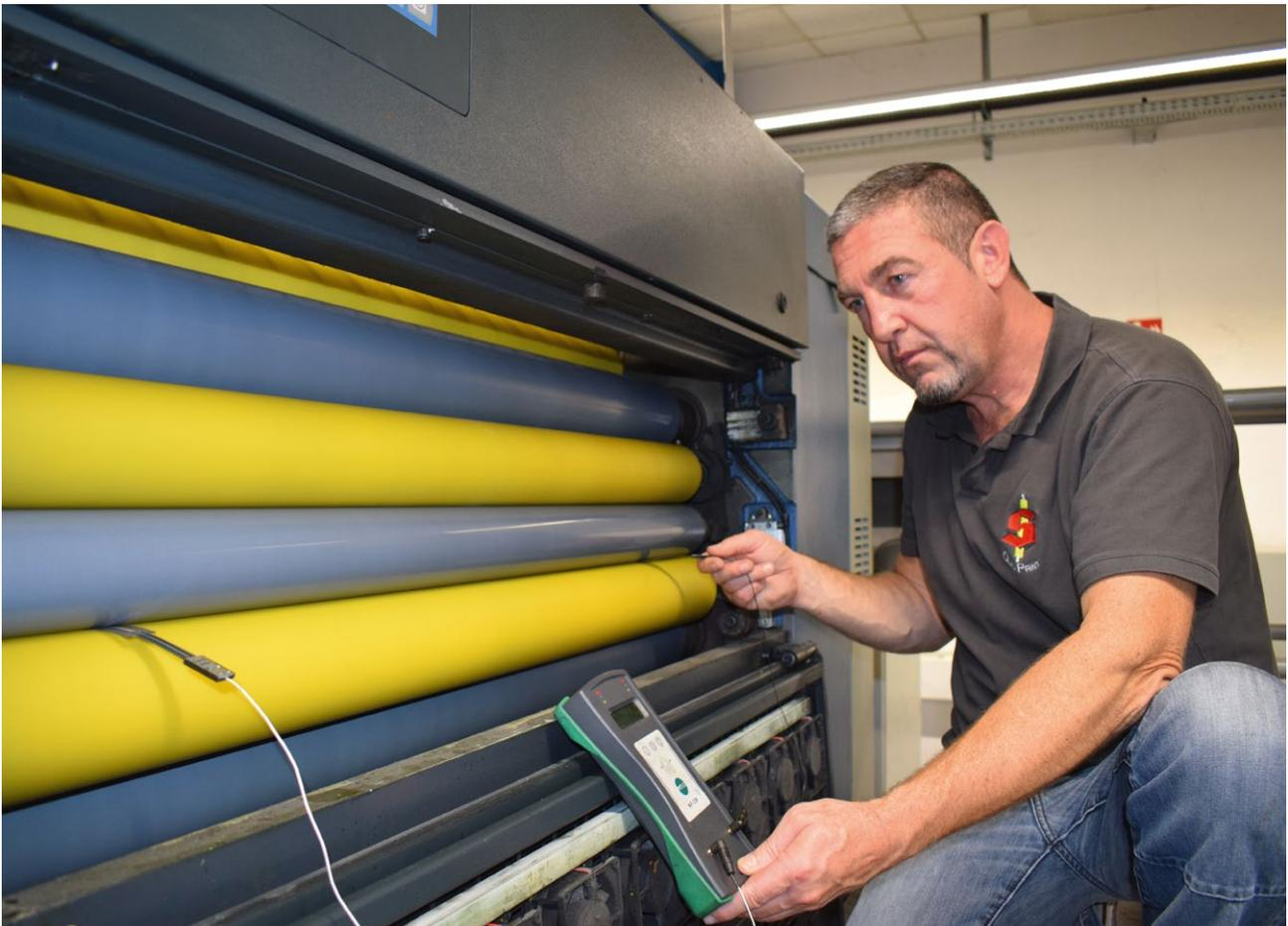
Adjustment of the DURAPRINT rollers with the NIP CON roller strip measuring device
